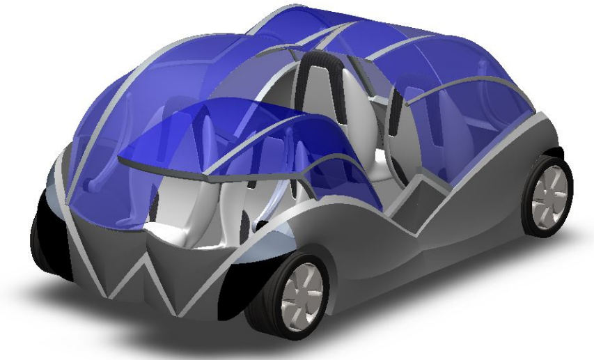
Fig. 8: Gullwing doors of concept vehicle. Design derived from courtesy of Kir Ari.
